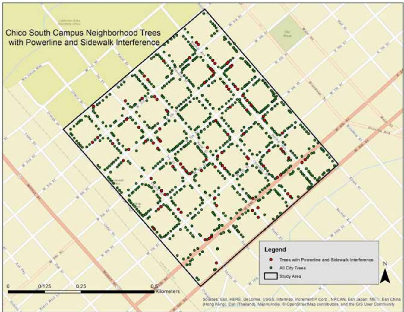
Figure 22: Location of trees that exhibit both powerline interference and sidewalk uplift in the study area.
