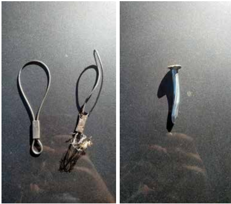
Figure 4: (Left) Unbroken and Broken Figure 8 loop tie (Right) Concrete Nail
