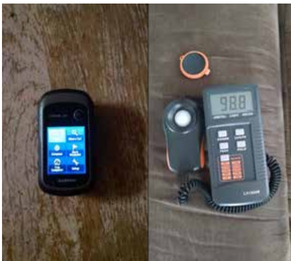
Figure 3. Primary data collection instruments; the LX1330B Digital Light Meter (left) and GARMIN etrex 30 (right)
