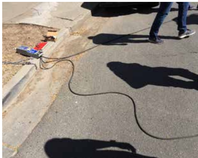
Figure 5. Metro-Count attached with pneumatic tubes being set up
