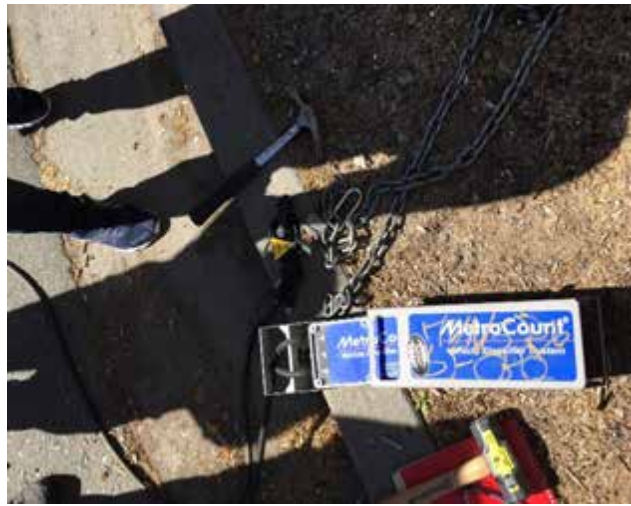
Figure 4. A Metro-Count device used for the traffic study
